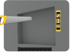
Measure and create the in-wall cutout for the mirror glass, ensuring the edges are straight and level.
