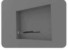
Install the cables and power supply needed for the television and ensure there is enough length to reach the television connectors. Tidy any excess length away to tidy the area (power supply, HDMI, aerial cable etc).
