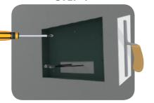
Slide the backbox into the cutout and fix into place with enough fittings to secure it. Ensure the box fits tight into the cutout and fill in any gaps around the edge of the backbox using a filler.
